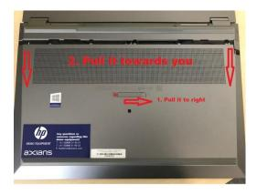
**Step 2.** Take of the battery off by clicking the two buttons to left simultaneously and pull battery out
