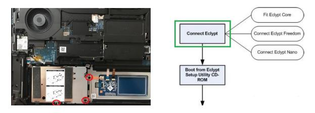
Step 4. Connect the Viasat Core Drive in the bracket as stated below
