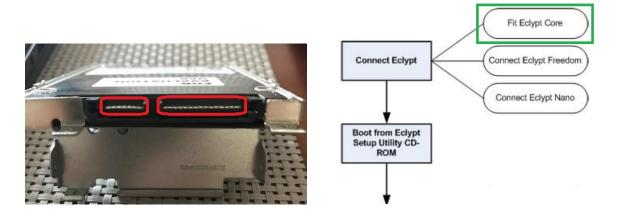
Step 5. Connect the Viasat Core 200 drive and close the cover
